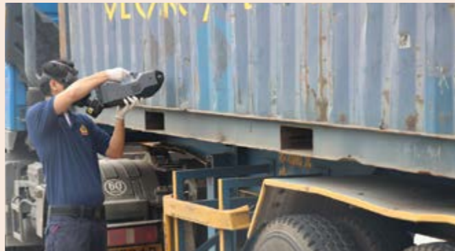
A Singapore Customs' Sea Export Team officer scanning the container with a handheld detector, to check for the presence of any toxic industrial chemicals.
