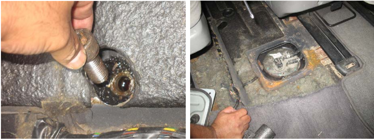
From left: The loose bolt that gave the game away; Top view of the modified fuel tank
